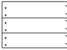
RP3 - ROOF PANEL - W2A01772 (1) 1 5/8"x15 5/8"x22" (42x396x558)
